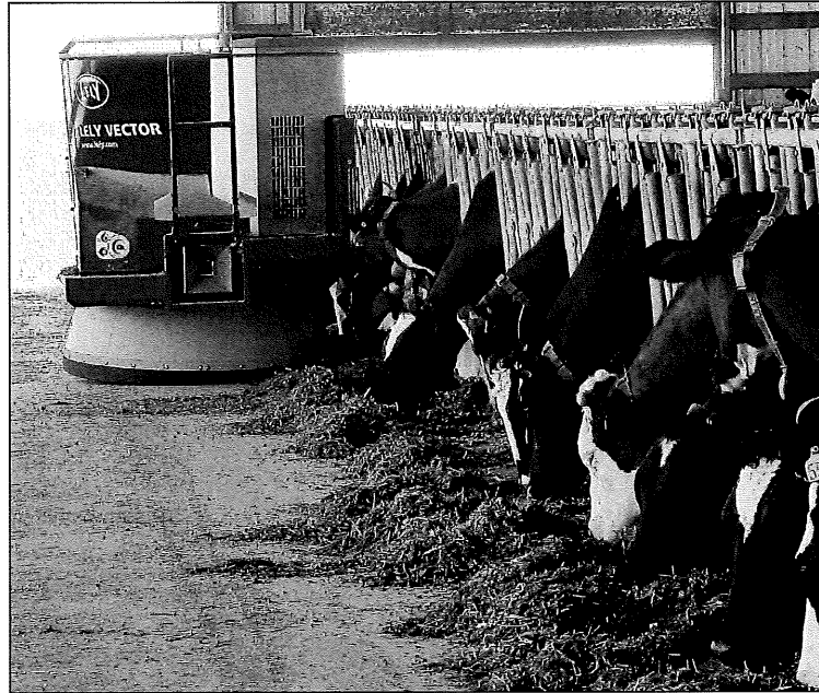
The Lely Vector pushes up the feed and measures how much feed is still in the bunker before putting down new feed. This helps it to keep the levels steady throughout the barn and avoid dumping large piles of remaining feed at the end of the barn.
