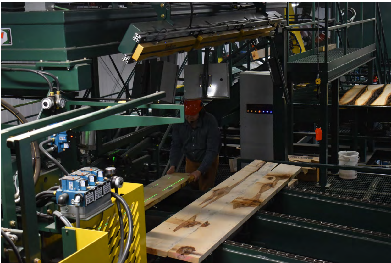
Logan Wells positions a board, using lasers to guide the cuts to its edges at Northcentral Technical College's Antigo campus. Rob Mentzer/WPR
