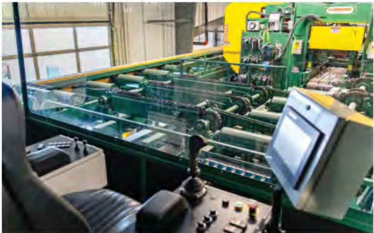
Students will practice secondary breakdown techniques and routing using a 54-inch horizontal resaw and preturning workstation.
