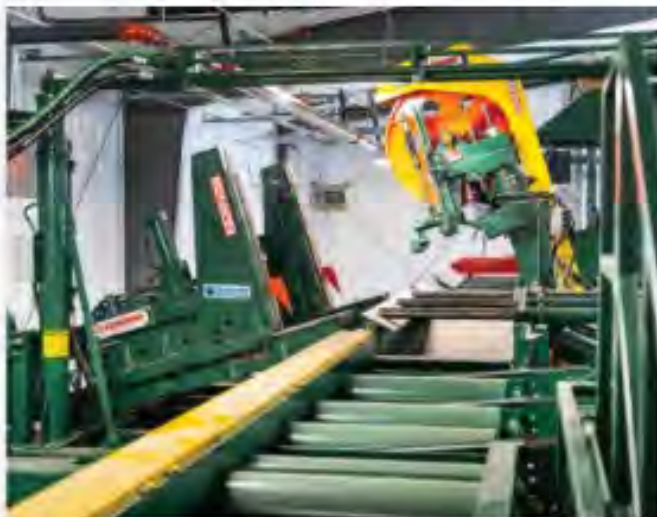
The Mill Technology Certificate program is taught on a sawmill provided and installed by Cleereman Industries and Cleereman Controls. Pictured here is Cleereman 54-inch double cut bandmill and linear tilt carriage.
