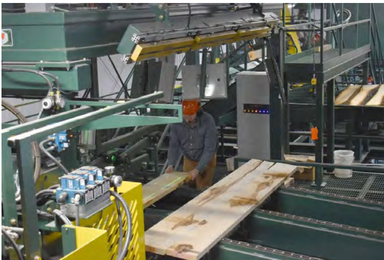
INSTRUCTOR LOGAN WELLS positions a board, using lasers to guide the cuts to its edges at Northcentral Technical College's Antigo campus. (Rob Mentzer/Wisconsin Public Radio)
