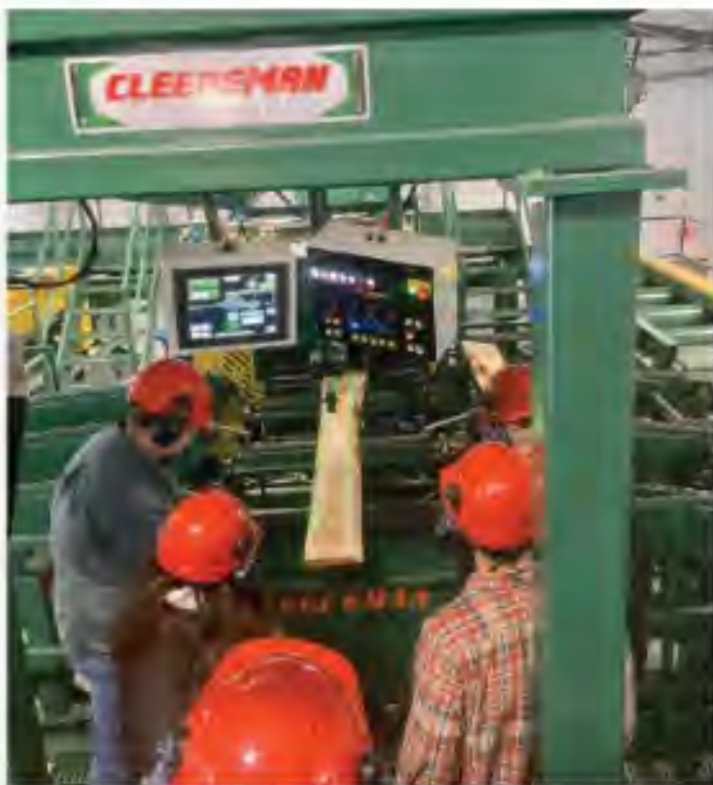
Throughout their time in the Mill Technology Certificate program, students will learn how to use an optimized two saw edger and practice edging lumber to acceptable wane limitations.
