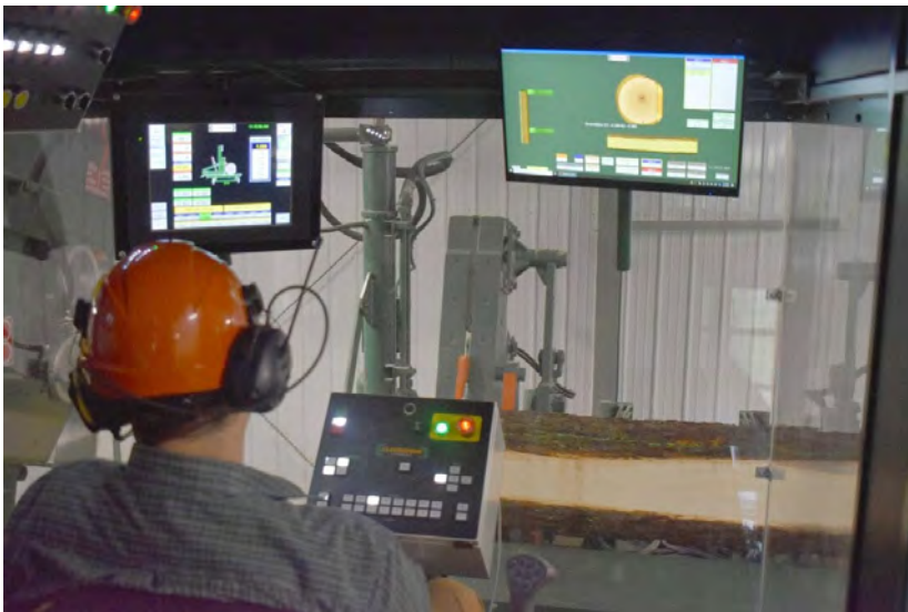
INSTRUCTOR LOGAN WELLS uses a scanner at Northcentral Technical College's Antigo, Wis., sawmill to determine the best cuts to make lumber out of a basswood log. (Rob Mentzer/Wisconsin Public Radio)
