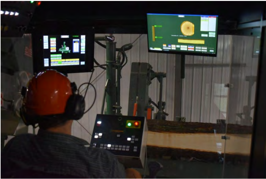
Instructor Logan Wells uses a scanner at Northcentral Technical College's Antigo sawmill to determine the best cuts to make lumber out of a basswood log. (Rob Mentzer / WPR)
